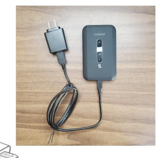
9. To turn on the hotspot press and hold the Power Button for 3 seconds.
