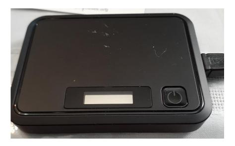
1. Plug in the AC adaptor to the wall outlet and the MicroUSB cable in the charging port.
