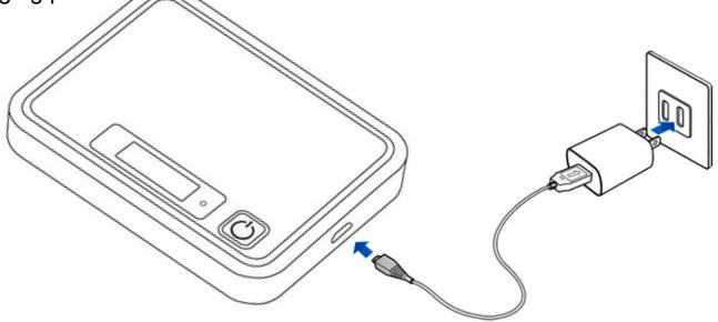
2. The indicator light on the power button illuminates red when charging starts. It may take up to three hours to fully charge the battery. The light will turn green when the device is fully charged.
